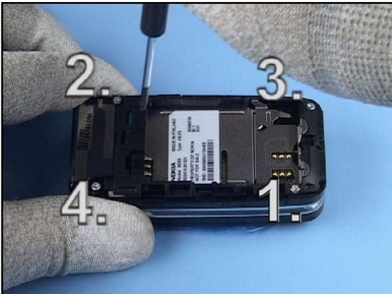
9. Unscrew the four screws in the order shown.
