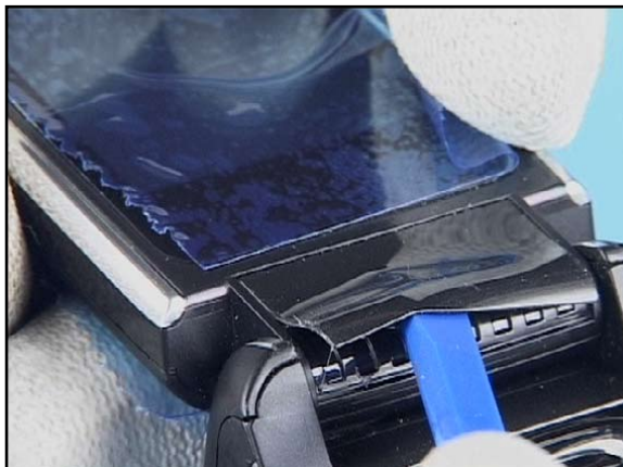
7. Complete the removal of the glued A-Cover Upper Bezel with the SS-93.
