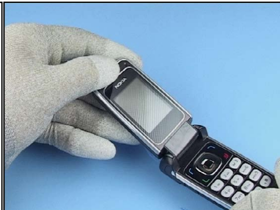
34. Check the window for cleanliness.
