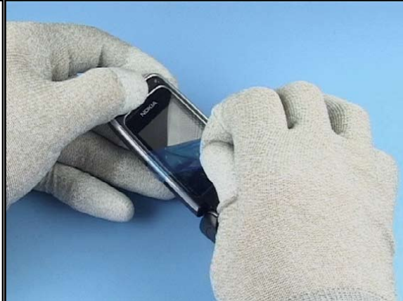
32. Remove the protective film from the LCD Window.
