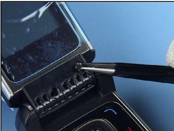
27. First insert the two screws with tweezers.
