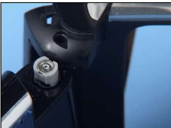
29. Hold the spring-loaded hinge pin down with your thumb while slowly separating one side of the hinge.
