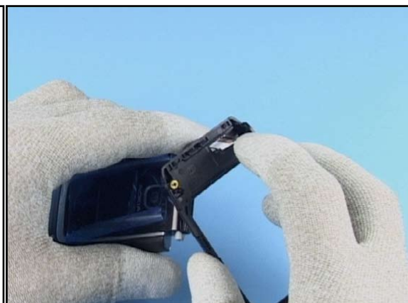
30. When separating the two parts, be very careful not to damage the Micro Coax Cable Assembly connector.
