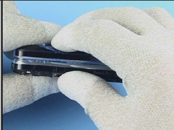
26. Close all the snaps and check that there are no gaps remaining.
