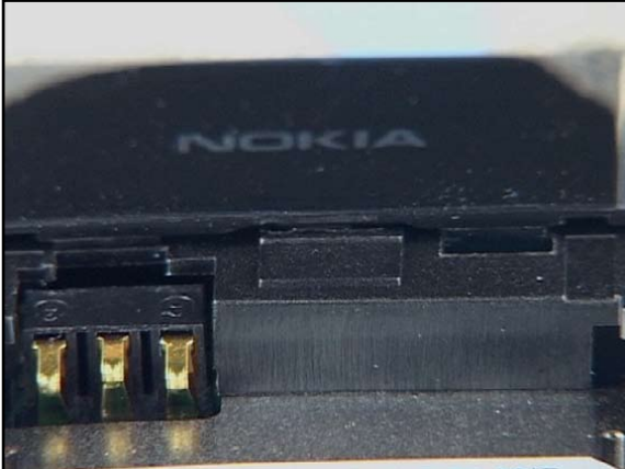
31. Turn the phone over and close the snap on the back.
