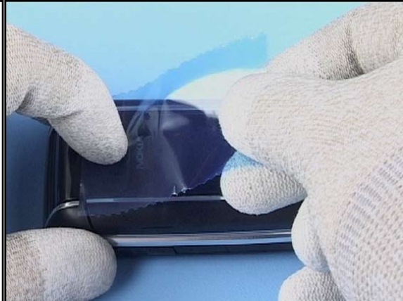
2. Cover the B-Upper Assembly window with protective film.
