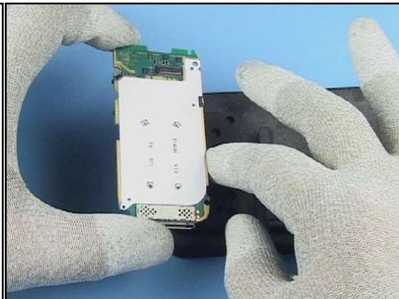
16. Finally check the correct positioning of the Domesheet on the Engine Module
