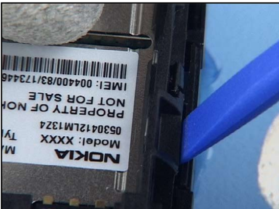
11. First, use the SS-93 to release the snap of the C-Cover Assembly on the Memory Card Door side.
