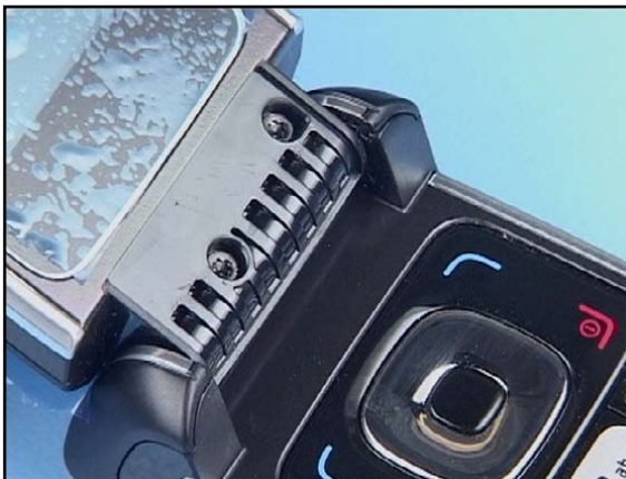
8. Ensure that no adhesive residue remains.
