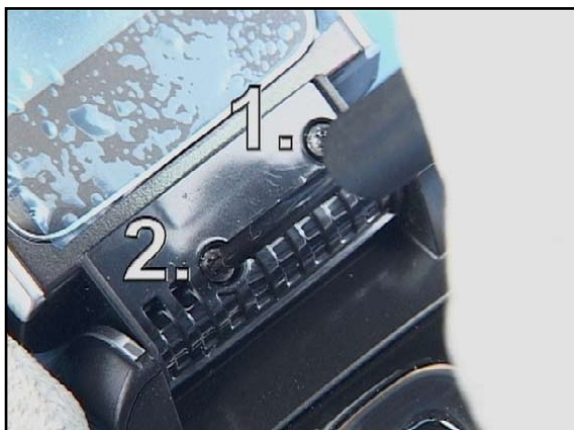
9. Unscrew the two screws in the order shown...
