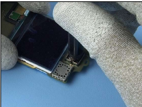
11. ... and press it smoothly into place with the back of the SS-45 camera removal tool.
