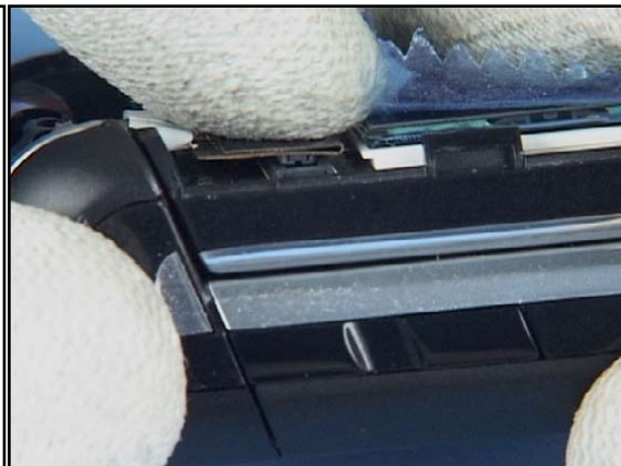
18. Close the Micro Coax Cable Assembly connector with your finger.
