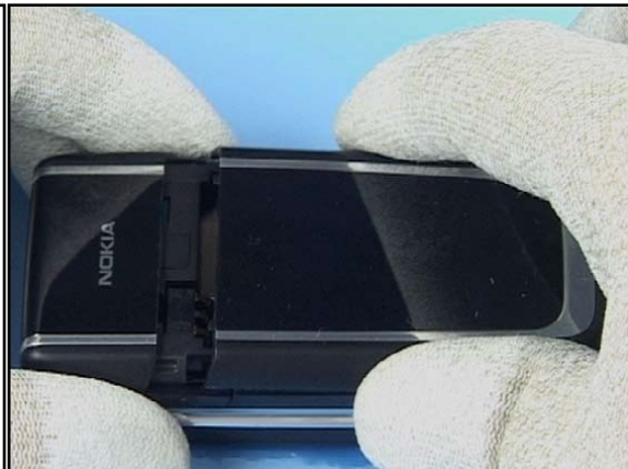
34. Complete the assembly by fitting the Battery Cover Assembly.
