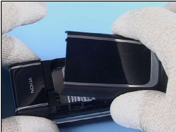
3. Unlock the Battery Cover and remove it.
