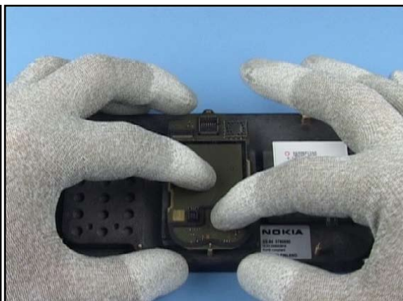
6. When the PWB Rigid is in the correct position, press it down on to the LCD AM.
