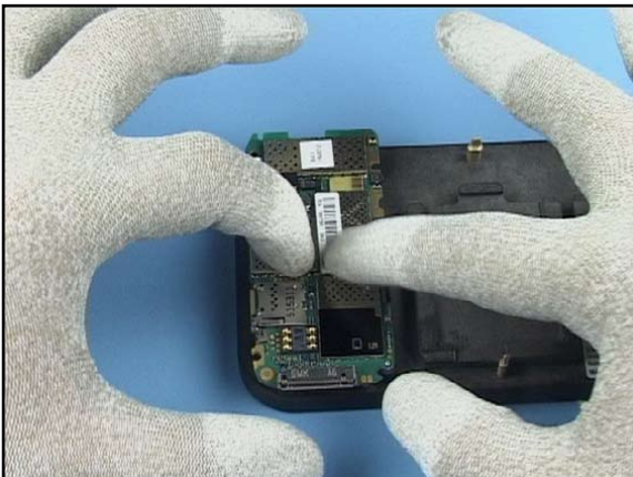
15. You can now press the Engine Module on to the Domesheet and remove the assembly.
