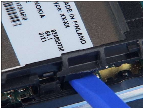
13. Now open the snap on the opposite side of the C-Cover Assembly.
