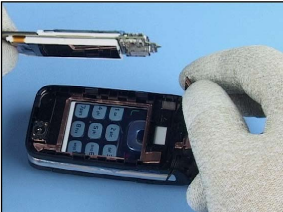
21. Remove the UI-Module and turn it over.
