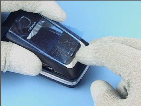
25. Start the assembly procedure at the pop port connector end.
