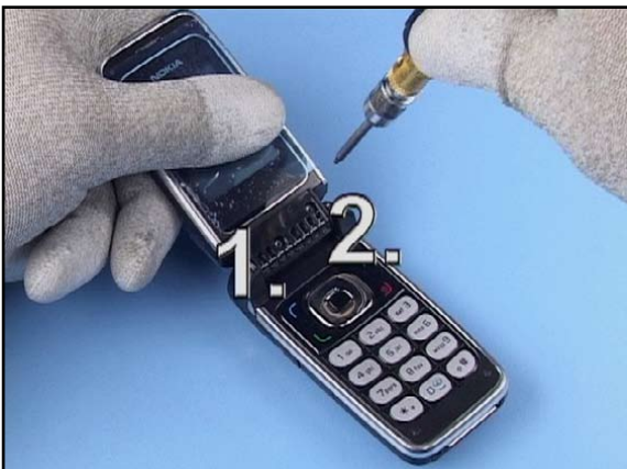
29. To avoid damaging the plastic threads, first turn the screws left to engage the thread and then tighten them lightly. Then, apply the correct torque in the order shown.
