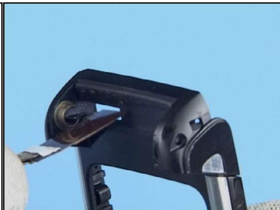
2. Feed the Micro Coax Cable Assembly connector through the slot in the A-Cover Assembly.
