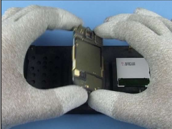
7. Remove the PWB Rigid include the LCD AM.
