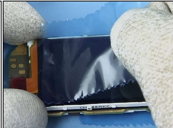
22. Cover the LCD AM with protective film.
