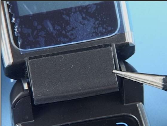
31. Use tweezers to work the A-Cover Upper Bezel into its correct position on the B-Upper Assembly...
