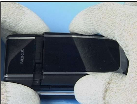
35. Complete the assembly by fitting the Battery Cover Assembly.
