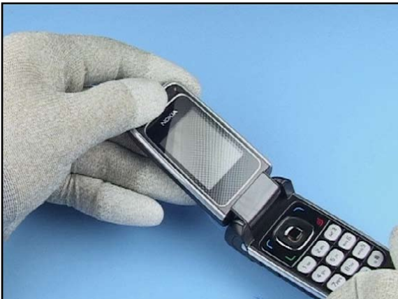
33. Check the window for cleanliness.
