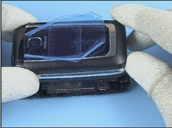
25. Take the unit and place it on to the C-Cover Assembly.
