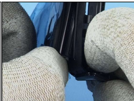
4. Depress the end of the Hinge Module and connect the parts. Ensure that the Hinge Module expands completely.
