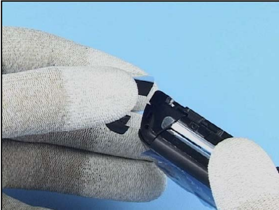
7. Remove the Antenna Cap...
