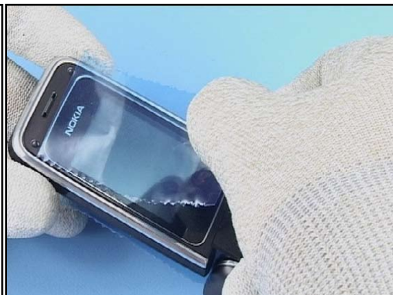
6. Cover the LCD Window with protective film.
