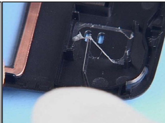
18. Remove all residual gasket adhesive.
