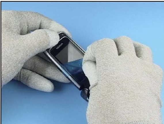
33. Remove the protective film from the LCD Window.
