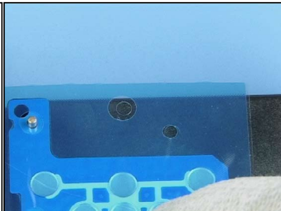
10. ... and upper left corners of the domesheet section
