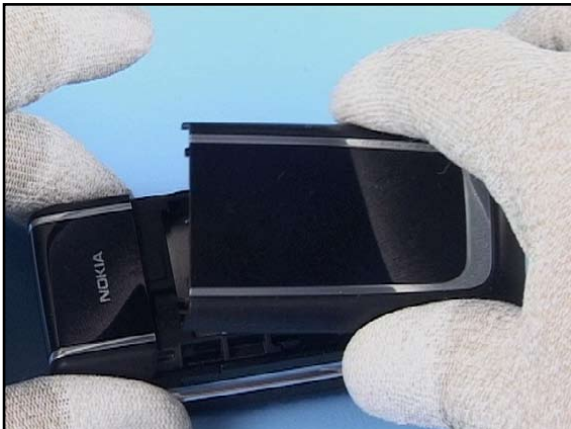
3. Unlock the Battery Cover and remove it.
