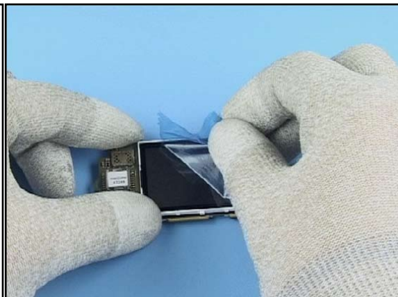
12. Remove the protective film from the LCD AM.
