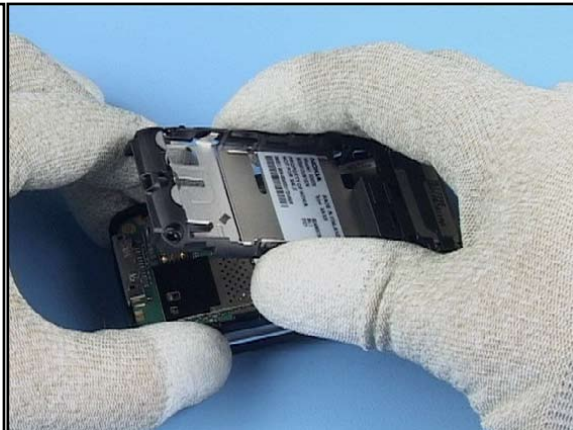
14. Remove the C-Cover Assembly starting from the Pop-Port Connector end.
