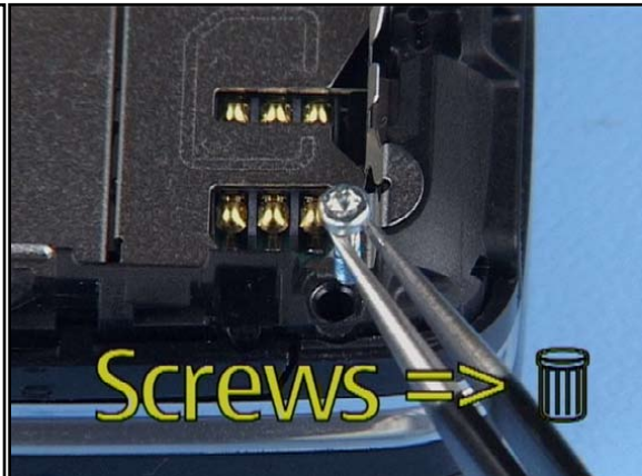
10. Remove the screws and discard them. These screws cannot be reused after disassembly.
