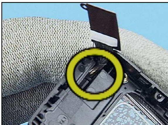
3. Be sure that the cable is correctly routed.
