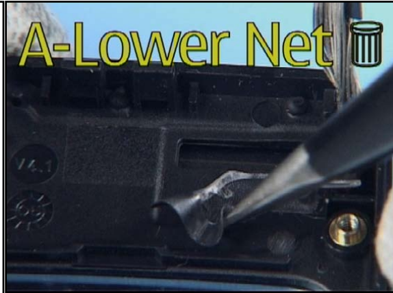
26. Remove the A-Lower Net with tweezers and discard it.
