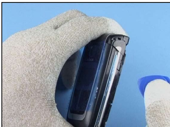
11. Release the snaps of the B-Upper Assembly with the SRT-6.
