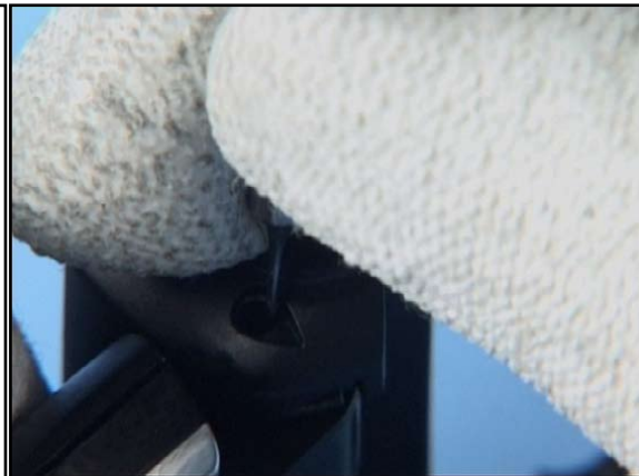
28. Pushing down on the tool will release the hinge.
