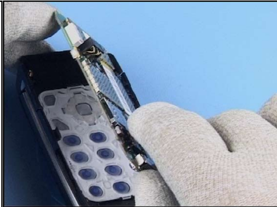
20. Raise the Engine Module slightly at the Pop-Port Connector end and then open it bookwise to a perpendicular position.
