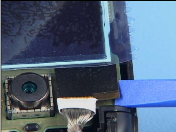
19. Open the Micro Coax Cable Assembly connector with the SS-93.
