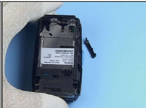
12. As the snap is released, the Memory Card Door automatically falls out and can be placed on one side.
