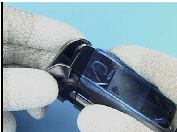
30. Put the Antenna Cap into position and close the snaps on both sides.
