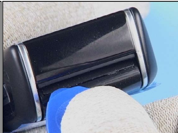
4. The A-Cover Upper Bezel is glued down. Begin to release the adhesion with the SRT-6 as shown.
