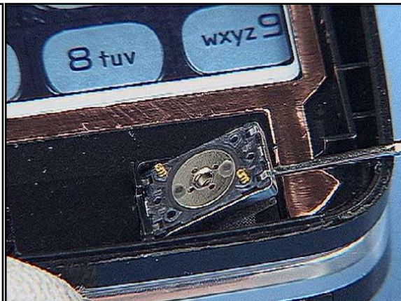
30. Remove the Earpiece with the dental pick.
