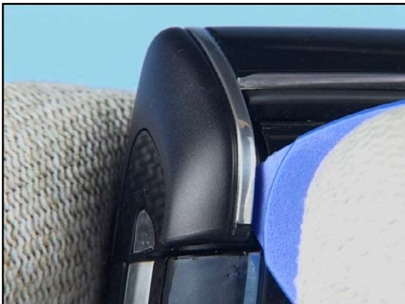
5. Release the snaps on the left side of the Antenna Cap with the SRT-6.
