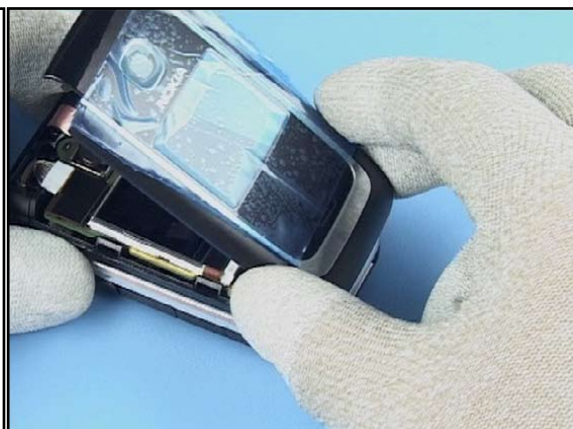
24. Place the B-Upper Assembly on the A-Cover Upper Assembly.
