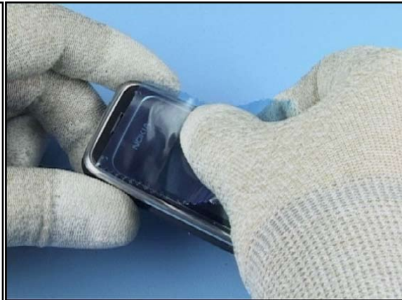
4. Cover the LCD Window with protective film.
